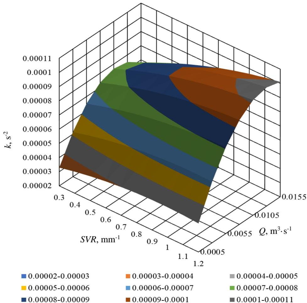
Fig. 2. Change in the coefficient of gasification rate depending on air supply and fuel sizes
